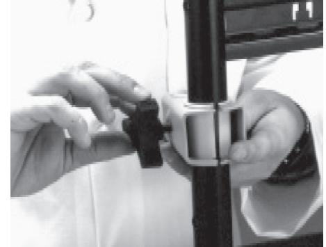
The plastic sleeves clip into the metal clamp halves. Snap the larger sleeve halves into the large recesses of the metal clamp. Squeeze the small sleeve halves together and install them into the front end of the clamp. Position the larger openings in the metal clamp around the Overbridge as shown. Insert the Carriage Bolt through the Clamp making sure the flats of the bolt head fit solidly into the square hole. Thread the knob onto the exposed bolt shaft and tighten to secure.
