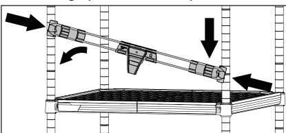
**Note:** PRL24-2S can be adjusted to fit shelves that are nominally 24" in depth or 24" in length.
