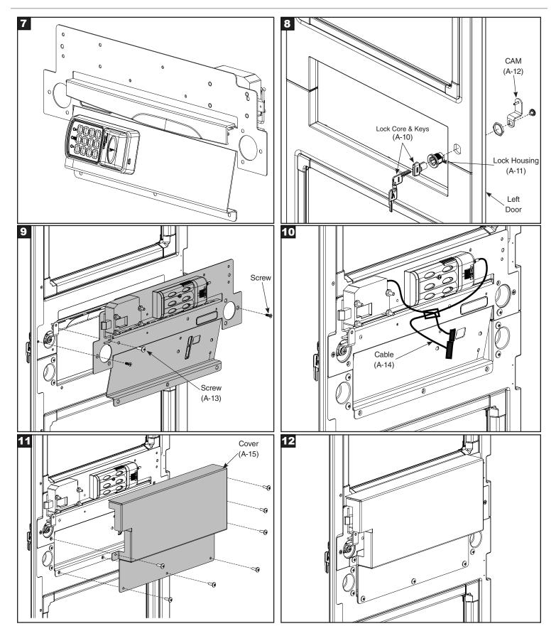
THIS COMPLETES ASSEMBLY OF BASIC PROXIMITY LOCKING ON DOOR
