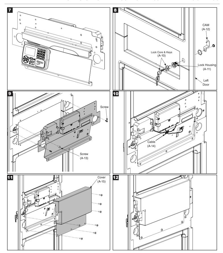
THIS COMPLETES ASSEMBLY OF ADVANCE AND WIRELESS PROXIMITY LOCKING ON DOOR
