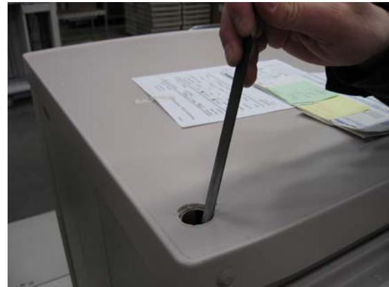
5. Take a sharpie and mark a line just below the mounting hole on the IV pole.
