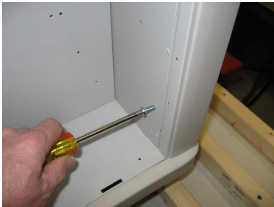
11. Use loktite<sup>®</sup> to secure the IV pole with 1/4 - 20 x 3/4 round head screw.
