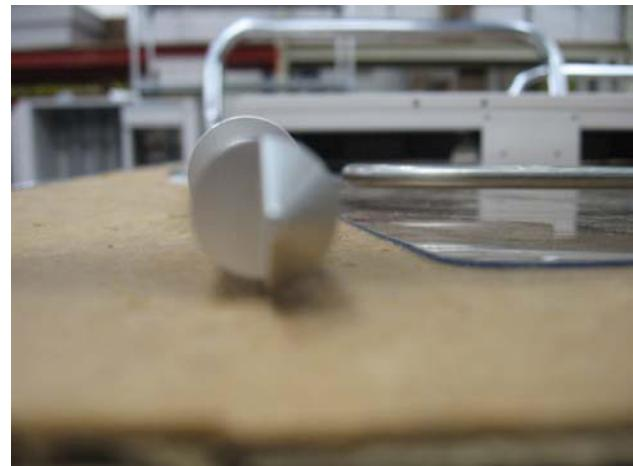
*Note: The D shape on the end of the IV pole. The hole at the bottom of the cart has a D shaped hole already in it.*
